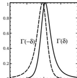
$$\Gamma(\delta) = 2g^2 \operatorname{Re} \left[ \int dt e^{-i\delta t - (\Gamma_\uparrow + \Gamma_\downarrow)t/2} \langle D_\alpha^\dagger(t) D_\alpha(0) \rangle \right]$$
