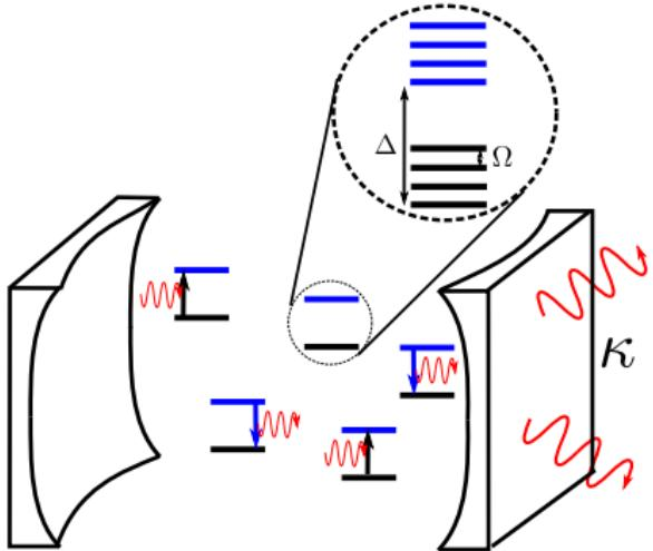
$$H_{\text{sys}} = \omega \psi^\dagger \psi + \sum_{\alpha} \left[ \frac{\epsilon}{2} \sigma_{\alpha}^z + g (\psi + \psi^\dagger) (\sigma_{\alpha}^+ + \sigma_{\alpha}^-) \right] + \sum_{\alpha} \Omega \left\{ b_{\alpha}^\dagger b_{\alpha} + \sqrt{S} \sigma_{\alpha}^z (b_{\alpha}^\dagger + b_{\alpha}) \right\}$$
