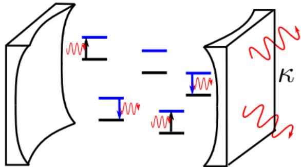
$$H_{\text{sys}} = \omega \psi^\dagger \psi + \sum_{\alpha} \left[ \frac{\epsilon}{2} \sigma_{\alpha}^z + g (\psi + \psi^\dagger) (\sigma_{\alpha}^+ + \sigma_{\alpha}^-) \right]$$
