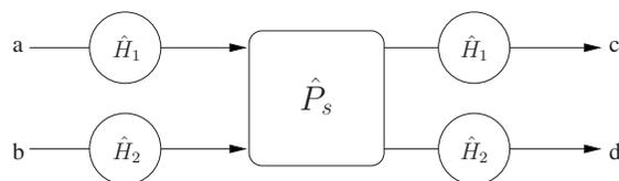
FIG. 1. A gate that uses a spin-parity measurement to measure the parity of  $S-T_0$  qubits. A pair of  $S-T_0$  qubits enters the gate in arms  $a$  and  $b$ . Each of the qubits is rotated by a Hadamard gate  $\hat{H}$ . The spin parity of the left spins [see Eq. (1)] from each qubit is then measured in the  $\hat{P}_s$  box. The qubits are rotated back by Hadamard gates and the parity of the spins is equivalent to the parity of the qubits.
