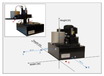
The Risø DA-15 and DA-20 OSL/TL reader, shown with the lid both open and closed. The figure shows the coordinates and positions of the external dose rate measurements listed below
