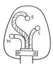
The earth wire is green and yellow stripes and must be connected to the terminal marked E.
