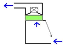
The filtered air is normally discharged into the atmosphere but in exceptional circumstances it is possible to recycle the air in the laboratory provided it has been passed through two HEPA filters and the procedure has HSE approval.
