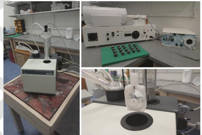
Fig. 3 The M3Ore Lab is equipped with (left) a KLY-5a Kappabridge with CSL cryostat and CS4 Furnace, (bottom right) a 3D automated rotator, and a selection of lab based and hand-held susceptibility meters, two impulse magnetisers, two isothermal tumbler demagnetisers (top right), two spinner magnetometers and a super cooled thermal demagnetiser housed in our new palaeomagnetic shielded room.
