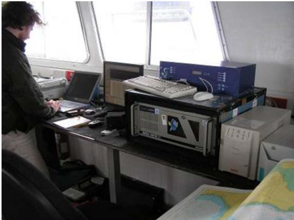
Figure 8: SEA/Submetrix SwathPlus bathymetric sidescan sonar
