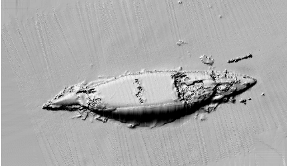
Figure 2 – Multibeam image of the Stirling Castle, Goodwin Sands, which sank in 1703 (ADU, University of St Andrews/ Reson Offshore Ltd)
