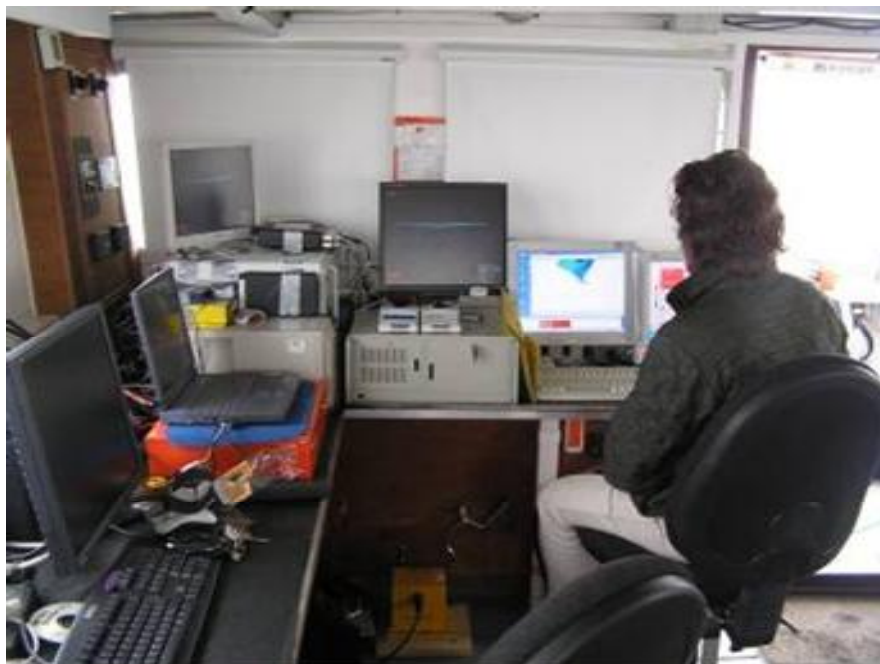
Figure 4.2: Reson 8125 Seabat multibeam system twin sonar head configuration and wheelhouse data acquisition hardware.
