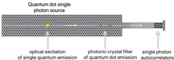
Electron micrograph of an example integrated quantum photonic device comprised of a on-chip quantum dot single photon source, a photonic crystal filter and an on-chip auto-correlation detector.
