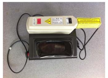
Figure 15. Example of UVC Mineral light with viewing box
