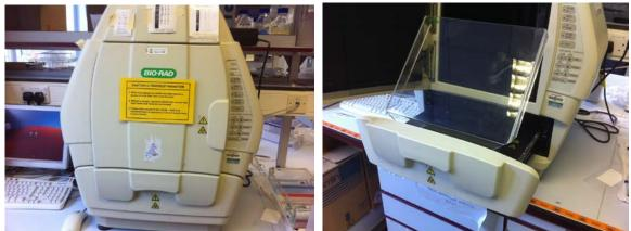
Figure 12. Bio-Rad Transilluminator Cabinet Figure 13. With 'Safety Screen' in place
