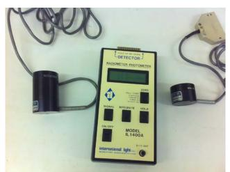
Figure 6. Solid State Radiometer with detectors
